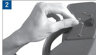
**STEP 2.** Gently insert a paper clip or similar object into the hole at the top of the tower, but DO NOT PRESS DOWN.
